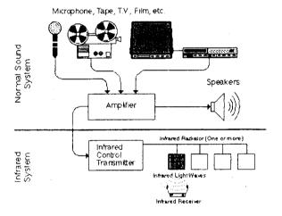
Figure A-3.8.3.7.B Infrared Sound Transmission System
